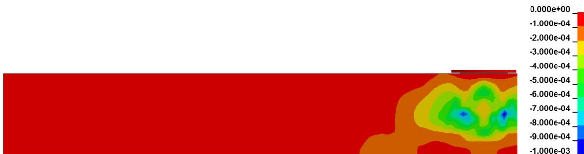
Figure 6.25 3<sup>rd</sup> principle strain (compression) 0.07 ms after impact.
